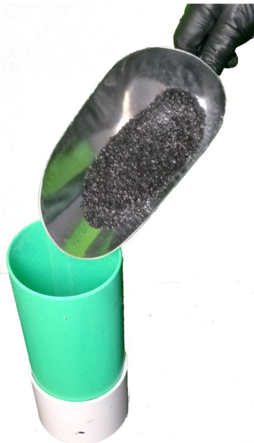
STEP 3: Add 2 cups of granulated carbon for lighter than water solvents and 4 cups for perc.
