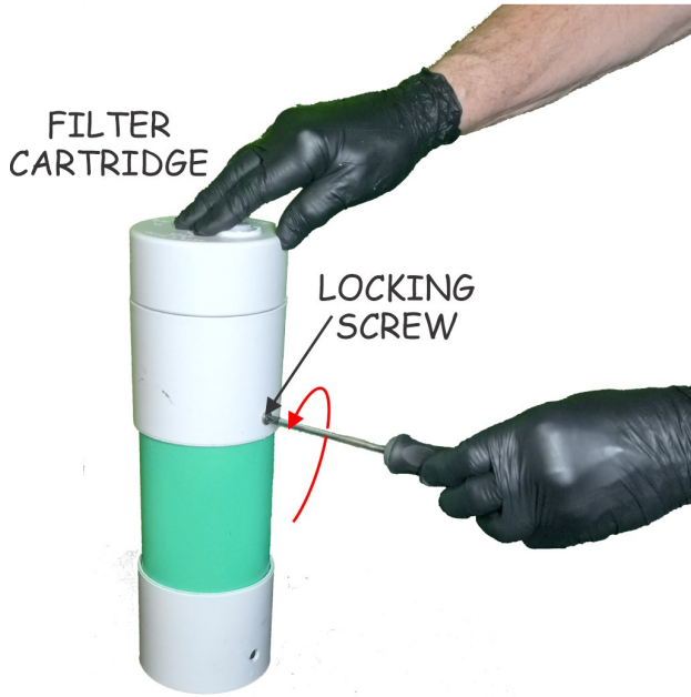
STEP 1: Unscrew locking screw from filter cartridge and place it where it won't get lost.
