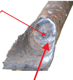
TOTALLY BLOCKED BOILER TUBE THAT ACTUALLY RUPTURED DUE TO OVERHEATING
