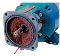
BUILD UP OF SCALE BEHIND PUMP IMPELLER
